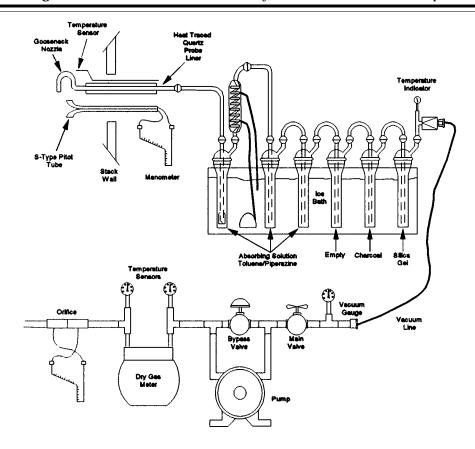
Figure 207-1-1. Sampling Train Configuration for Isocyanates
