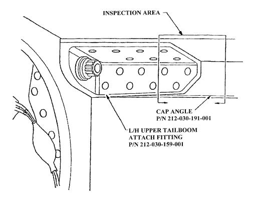
Figure 1 Fuselage Tailboom Attachment Inspection
