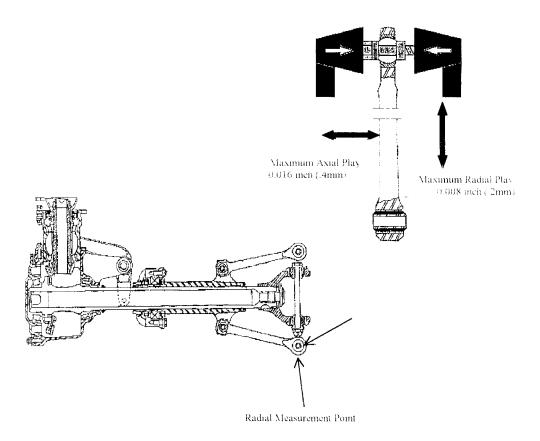
Figure 2. Play Measurement on Tail Rotor Pitch Control Rod
