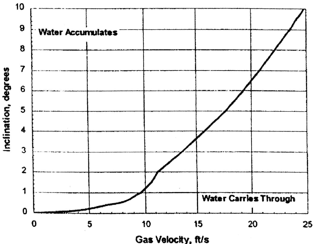
*Simple spreadsheet to calculate critical angle for liquid hold-up. Line diameter, pressure, and temperature are data inputs.*
