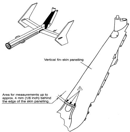
Measurements are to be taken at at least three locations on the skin panel of the vertical fin. Care has to be taken that the external calipers are held squarely to the skin panel wall while measurements are being taken, since tilting of the calipers can lead to false results. If the panel thickness, including the primer coating, is at least 0.778 mm (0.03063 inch) at every measured location, no further action is necessary.
