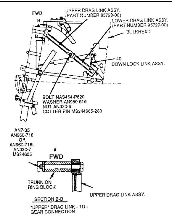
**Note 1:** Paragraph 2. Modified Components of the INSTRUCTIONS section of The New Piper Aircraft, Inc. Service Bulletin No. 1123A, dated November 30, 2004, specifies modified parts that you may install for improved service life.
