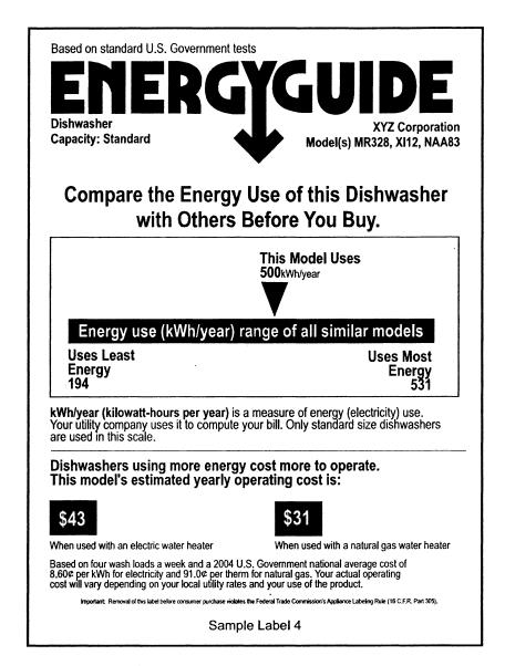
FIGURE 1 - (Current EnergyGuide Label - Sample)
