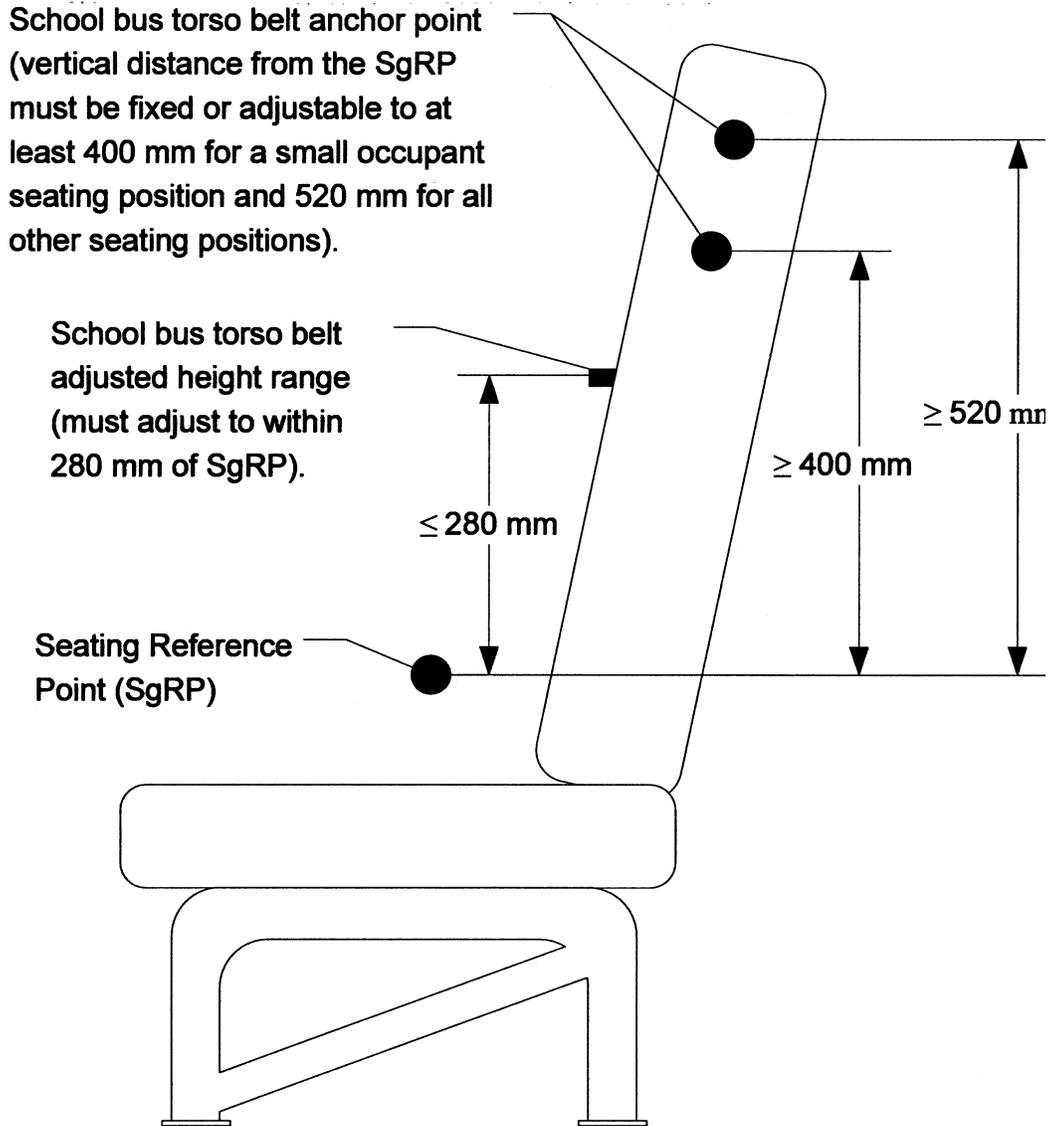
**Figure 1—Seat belt anchorage diagram**
