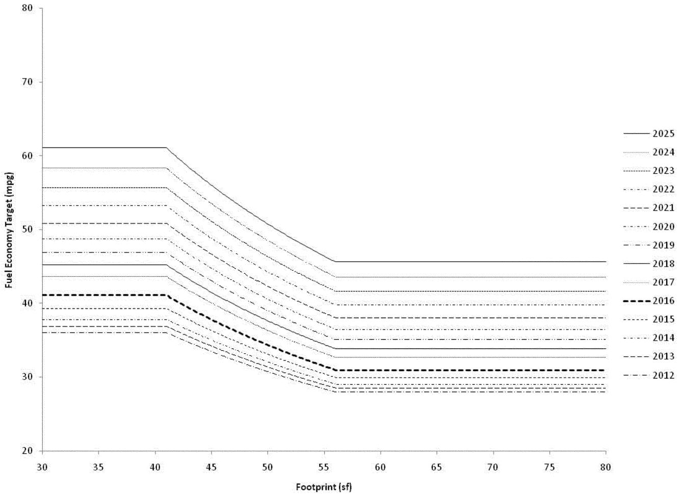
Figure I-2 CAFE Target Curves for Light Trucks
