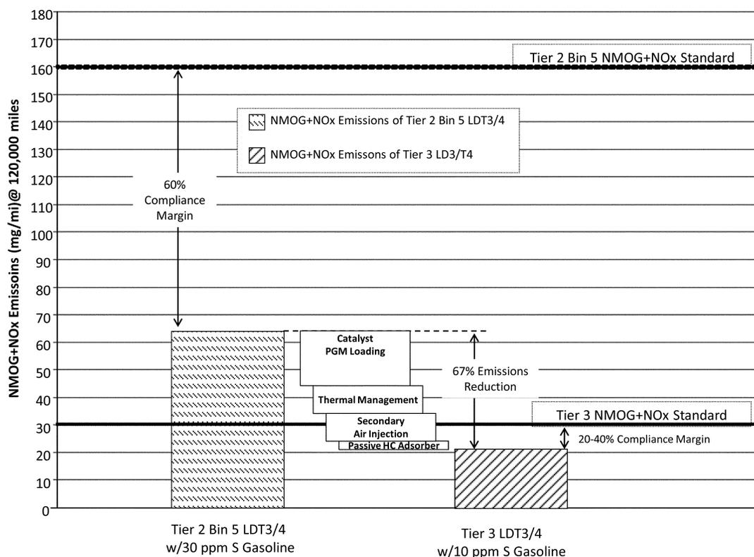
**Figure IV-1: Contribution of Tier 3 Technologies to Large Light-Duty Truck Compliance<sup>261</sup>**
