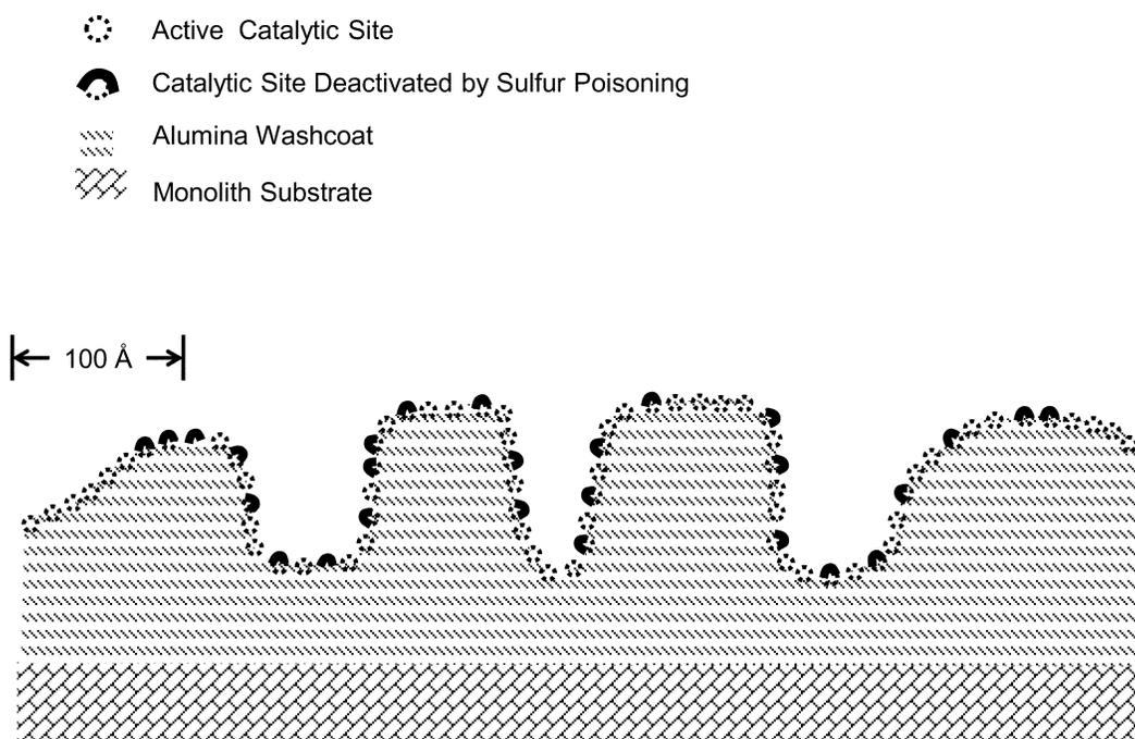
**Figure IV-2 Functional schematic showing selective poisoning of active catalytic sites by sulfur compounds. Adapted from Heck and Farrauto 2002.<sup>280</sup>**
