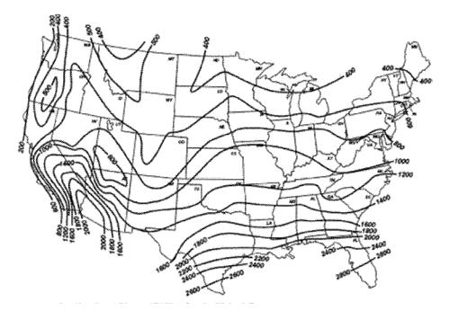
Figure 2—Cooling Load Hours (CLH<sub>A</sub>) for the United States
