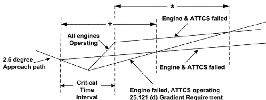
\* The engine and ATTCS failed time interval must be no shorter than the time interval from the point of simultaneous engine and ATTCS failure to a height of 400 feet used to comply with 125.2(b) for ATTCS use during takeoff.
