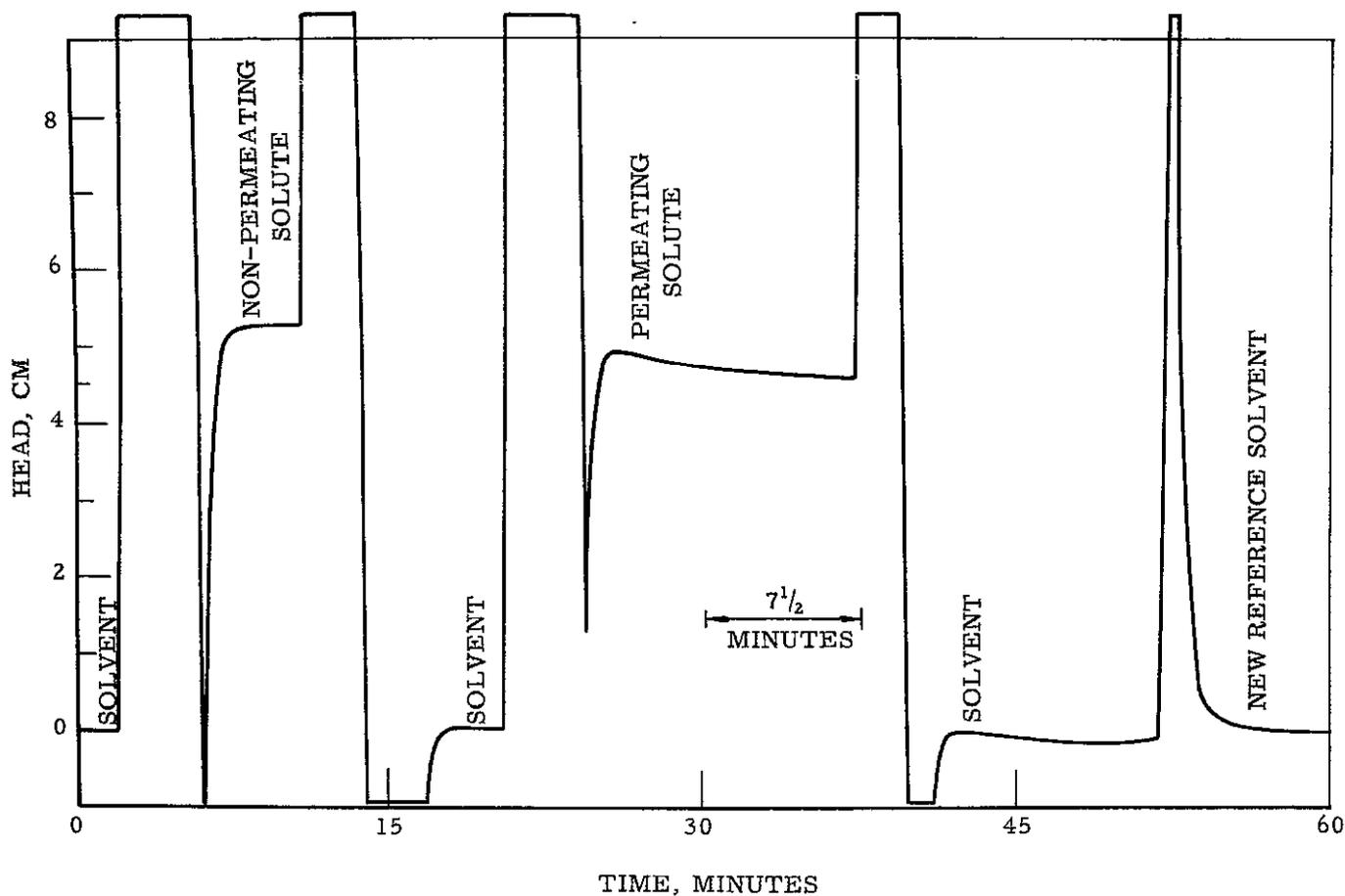
Figure 3 — Typical Recorder Chart (Continuous Chart Drive)
